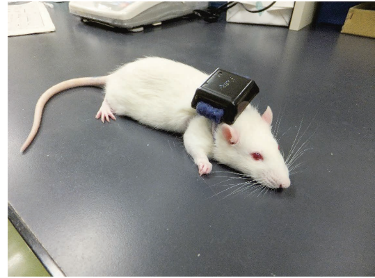
Fig. 1. Installation of the actigraphy device. A rat carries the actigraphy device on their back, secured with an elastic belt.
