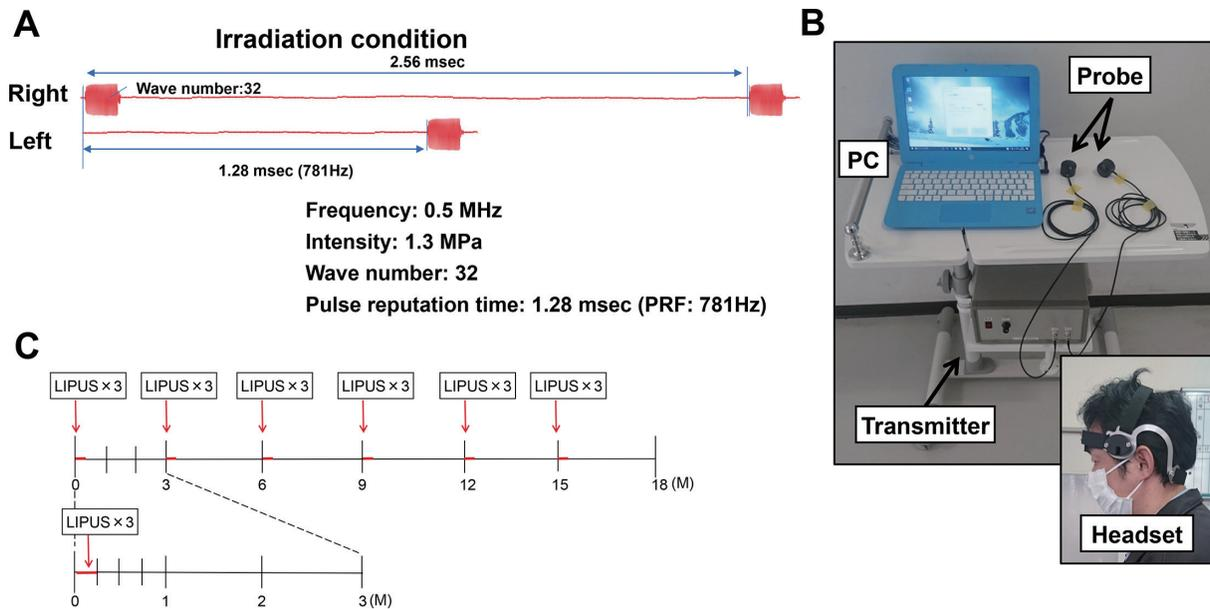
Fig. 1. Whole-brain low-intensity pulsed ultrasound (LIPUS) therapy for Alzheimer's disease.
